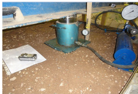
Figure 6. Other equipments for plate loading test
