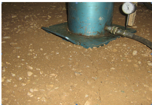
Figure 3. Plate loading test on soil without shred tire
