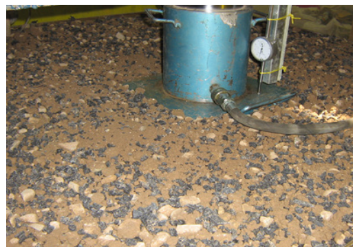
Figure 4. Plate loading test on soil mixed with 10% shred tire
