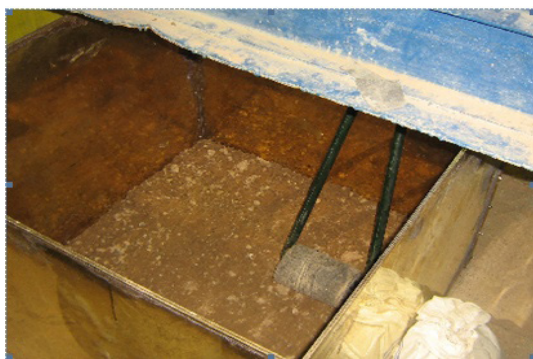
Figure 5. Loading box for plate loading test
